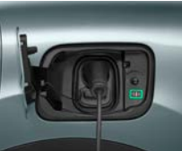
Charge Complete Mode (Constant green LED)
