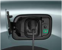
Charging Mode in Progress (Flashing green LED)
