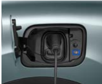
Deferred Charge Mode (Flashing blue LED)
