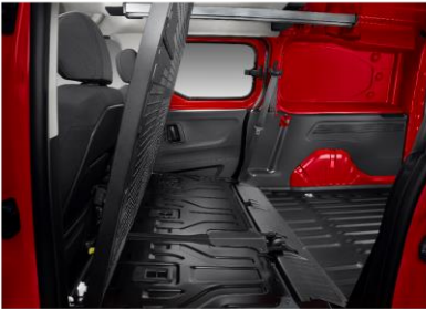
Crew Cab Seats folded almost flat with Bulkhead slid forwards
