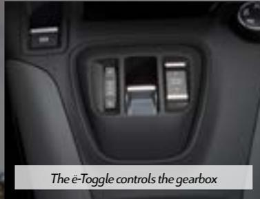
*The e-Toggle controls the gearbox*
