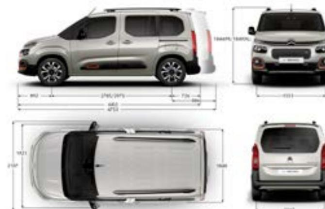
Measurements in millimetres.
