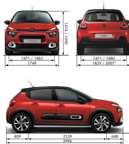
\* Vehicle width/width with door mirrors. All measurements are in millimetres.
